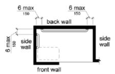
Figure 608.3.3 Grab Bars for Alternate Roll-In Type Showers
