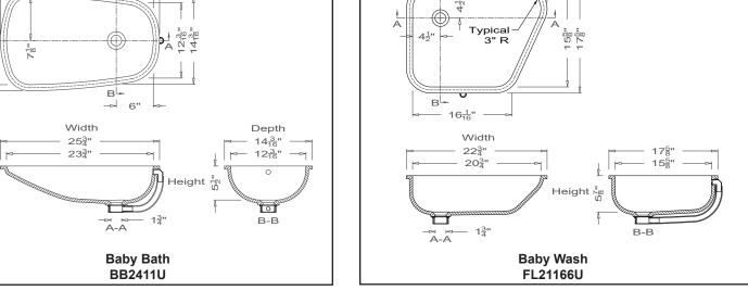
All drain holes are nominally 1 3/4" in diameter and accept all standard drain hardware, including waste overflow units if required.
