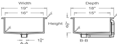
All drain holes are nominally 1  $\frac{3}{4}$ " in diameter and accept all standard drain hardware.
