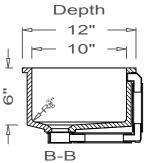
All drain holes are nominally 1  $\frac{3}{4}$ " in diameter and accept all standard drain hardware.
