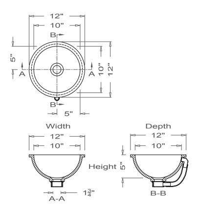
All drain holes are nominally 1  $\frac{3}{4}$ " in diameter and accept all standard drain hardware.
