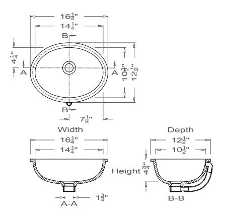
All drain holes are nominally 1  $\frac{3}{4}$ " in diameter and accept all standard drain hardware.
