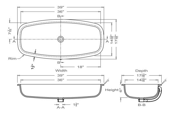
All drain holes are nominally 1  $\frac{3}{4}$ " in diameter and accept all standard drain hardware.
