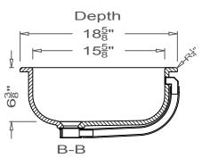
All drain holes are nominally 1  $\frac{3}{4}$ " in diameter and accept all standard drain hardware.
