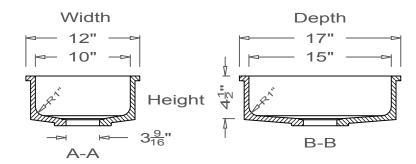
This Kitchen Sink is prepared for a standard  $3\frac{1}{2}$ " basket strainer drain assembly.
