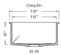
This Kitchen Sink is prepared for a standard  $3\frac{1}{2}$ " basket strainer drain assembly.
