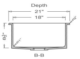
This Kitchen Sink is prepared for a standard  $3\frac{1}{2}$ " basket strainer drain assembly.
