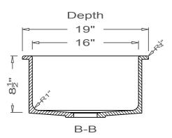
This Kitchen Sink is prepared for a standard  $3\frac{1}{2}$ " basket strainer drain assembly.
