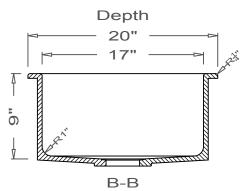
This Kitchen Sink is prepared for a standard  $3\frac{1}{2}$ " basket strainer drain assembly.
