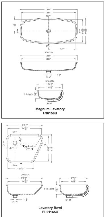
Grifform Innovations<sup>®</sup> has developed many style options of lavatory bowls. These bowls are prepared for ease of installation. All drain holes are nominally 1<sup>3</sup>/<sub>4</sub>" in diameter and accept all standard drain hardware, including waste overflow units. All lavatory drains come with an overflow drain assembly unless requested otherwise.
