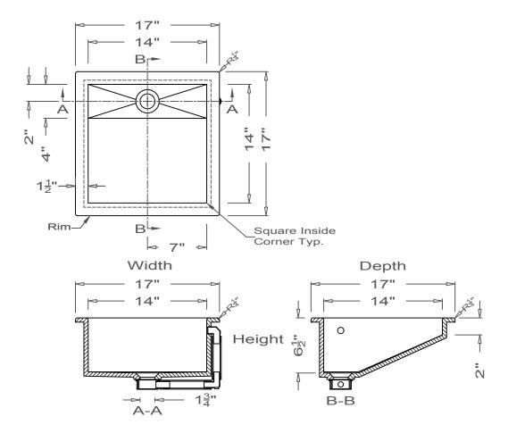
All drain holes are nominally 1  $\frac{3}{4}$ " in diameter and accept all standard drain hardware.
