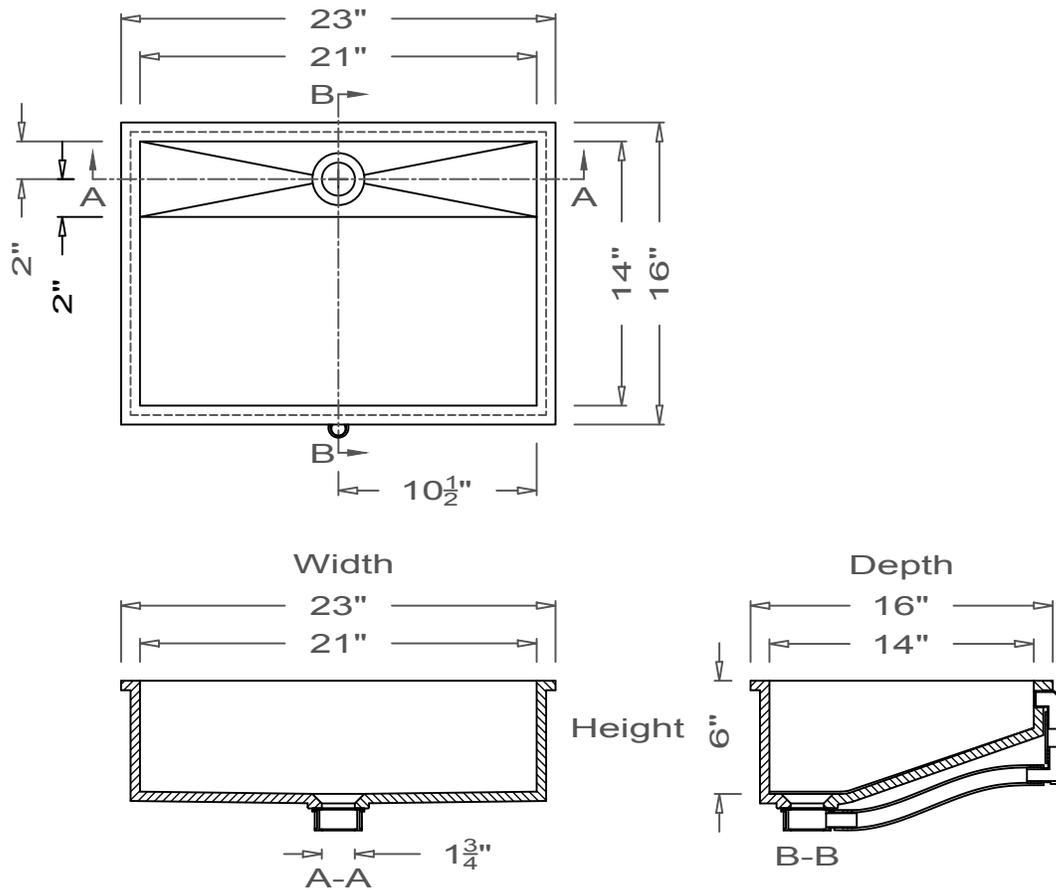
All drain holes are nominally 1 3/4" in diameter and accept all standard drain hardware.
