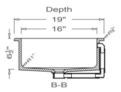
All drain holes are nominally 1  $\frac{3}{4}$ " in diameter and accept all standard drain hardware.
