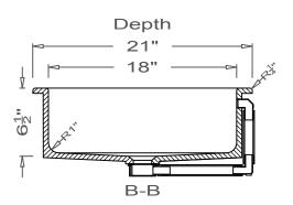
All drain holes are nominally 1  $\frac{3}{4}$ " in diameter and accept all standard drain hardware.
