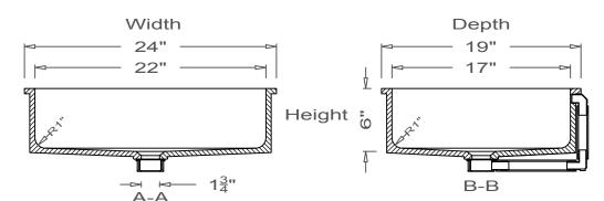
All drain holes are nominally 1  $\frac{3}{4}$ " in diameter and accept all standard drain hardware.
