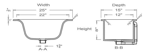
All drain holes are nominally 1  $\frac{3}{4}$ " in diameter and accept all standard drain hardware.
