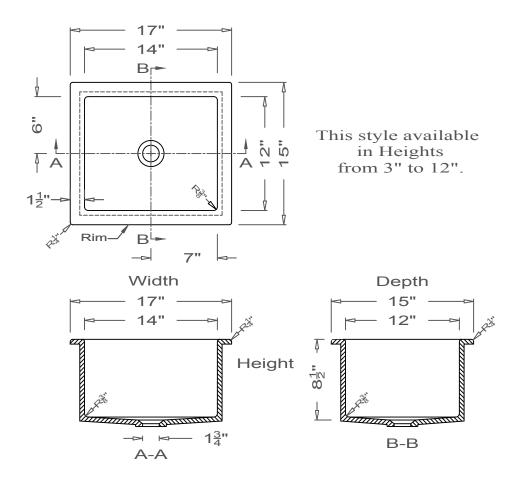
All drain holes are nominally 1  $\frac{3}{4}$ " in diameter and accept all standard drain hardware.
