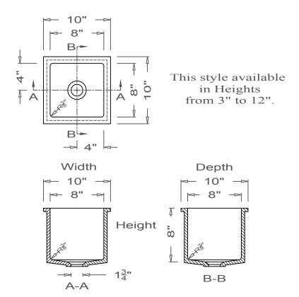
All drain holes are nominally 1  $\frac{3}{4}$ " in diameter and accept all standard drain hardware.
