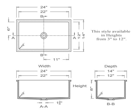
All drain holes are nominally 1  $\frac{3}{4}$ " in diameter and accept all standard drain hardware.
